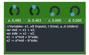
This is a mid-side plugin (operating on the first 2 inputs). You can control the amount of mid and side signal with the parameter sliders "a" and "b". Note how you can define additional local variables by
