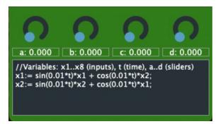
This is a set of formulas that lets the left and right channel (again, this example is for the first two inputs only, but everything can easily be extended to the rest) with a certain frequency. Note the use of the value of the time parameter, "t".
