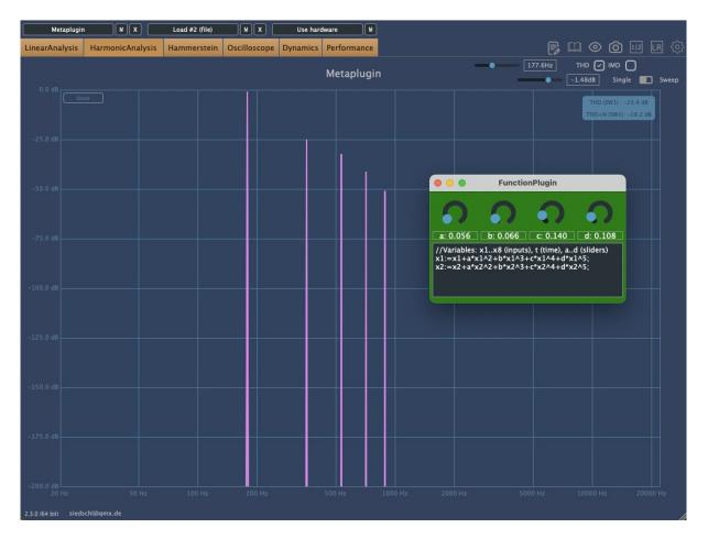
Using the powers  $x^2$ ,  $x^3$ ,  $x^4$  and  $x^5$ , you can adjust the contributions of harmonics to the input signal with the 4 parameters a, b, c and d.
